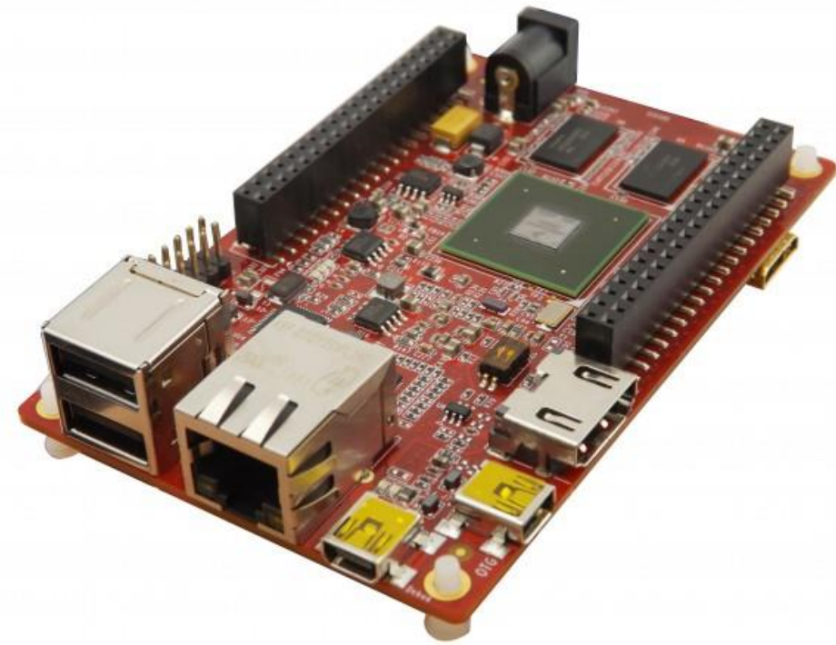
MarS Board Freescale i.MX6 Dual Processor Development Board
